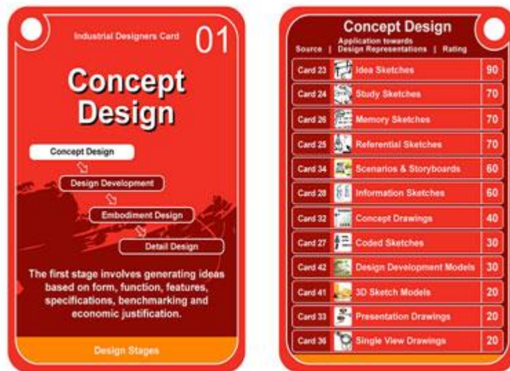
Figure 3. Sample card from the industrial design set for the design stage section, showing information on concept design.
